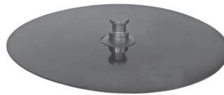
Fifth Wheel Disk shown with King Pin
